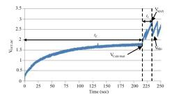
Fig. 12. Cold start duration time (tc) and charging time (tr) at the port of the storage capacitor [50].
