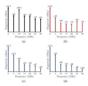
Fig. 3. Harmonic balance for the detector (a) without LPF, (b) with LPF, (c) with tunable LPF (bias: +8 V), and (d) with tunable LPF (bias: 0 V) [26].
