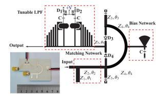
Fig. 2. Envelope detector and rectifier circuit with a tunable LPF structure [26].
