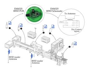
Fig. 26. Wireless and passive digital I/O digitization using EM4325 advance RFID tag and energy harvesting.
