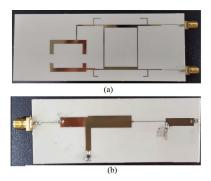
Fig. 6. (a) Antenna and asymmetrical coupler. (b) Fabricated sample of the rectifier circuit [37].
