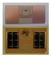
Fig. 23. Solar energy harvesting prototype to improve the passive RFID tag reading range: (a) original tag and (b) modified tag with oscillator circuit and solar cells [91].
