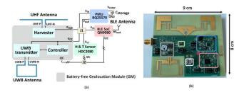
Fig. 20. (a) Schematic of the battery-less UWB BLE tag. (b) Prototype of BLE tag [80].
