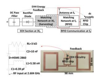
Fig. 22. System setup of RF energy harvesting using third harmonic to increase reading range of passive RFID [88].
