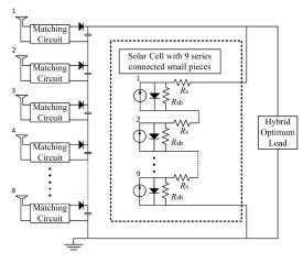
Fig. 15. Proposed dc combining circuit model of the hybrid RF-solar energy harvester [60].
