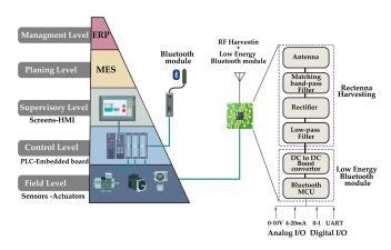
Fig. 25. Automation pyramid data flow and RF Energy harvesting data acquisition block diagram.
