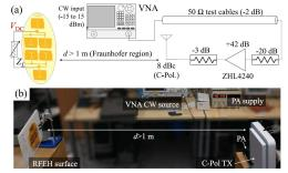
Fig. 9. (a) Block diagram for measuring rectenna performance. (b) Photograph of the experimental/measurement setup [42].
