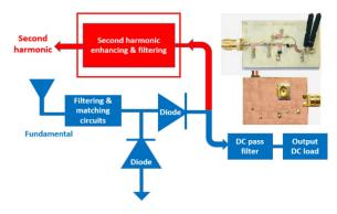
Fig. 7. Proposed block diagram of harmonic feedback rectifier [41].
