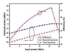
Fig. 8. Effect of harmonic power and conversion efficiency with respect to input power level [41].
