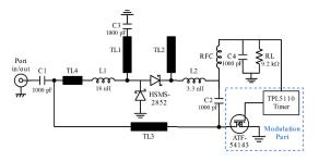
Fig. 10. Schematic of the proposed single-port harmonic transponder with modulation capability [43].
