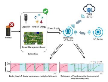
Fig. 21. Ambient light energy harvesting setup and data latency improvement by avoiding restarting the BLE node [82].
