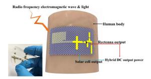
Fig. 14. Proposed flexible hybrid (solar + RF) energy harvesting circuit and a photograph of experimental setup on the human phantom [57].
