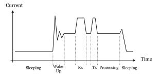
Fig. 19. BLE chipset duty cycle current consumption pattern.
