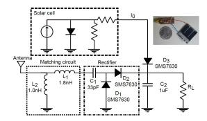
Fig. 13. Circuit diagram of the hybrid RF solar harvester and a photograph of the complete harvester prototype [53].
