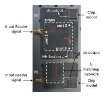
Fig. 24. Two RF energy harvesting prototypes using EM-4325 RFID chip. (a) Augmented tag that uses the chip model. (b) Chip model [103].
