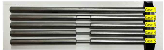
Fig. 12. Specimens for the indoor experiment (SS400 cylindrical steel rod).
