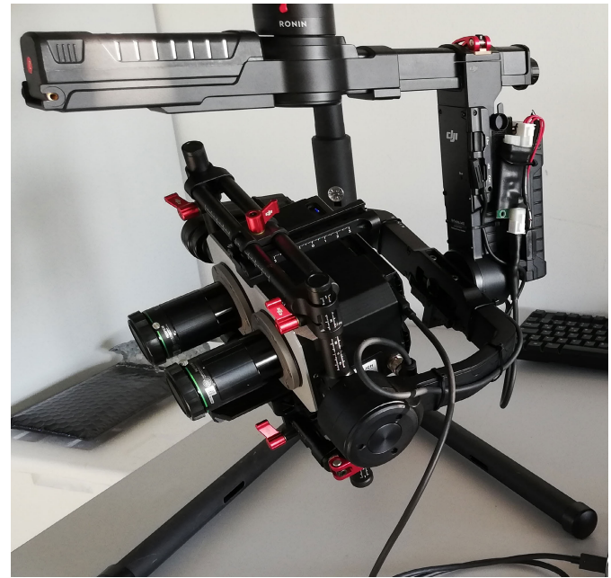
Fig. 5. SIF dual-camera system mounted on a DJI Ronin MX gimbal, capable of powering cameras via additional gimbal battery.
