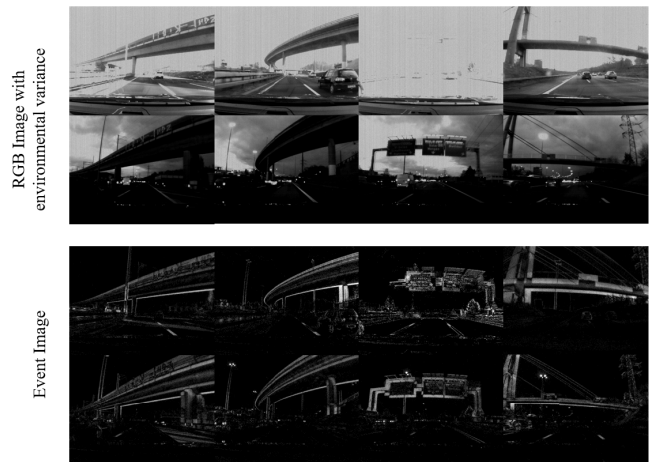
Fig. 1. Sample images from the DDD17 dataset taken from conventional cameras and event cameras. Even though they were taken in the same area and time of day, intensity images are sensitive to changes in illumination (first and second columns), and problems arise when the light is too bright or dark (third and fourth columns). However, the camera is more robust against these problems.
