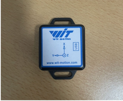
Fig. 4. Gyro sensor used for measuring face direction during training data acquisition.
