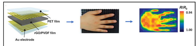
Fig. 4. Schematic of rGO/PVDF temperature sensor showing temperature distribution on human palm [61].
