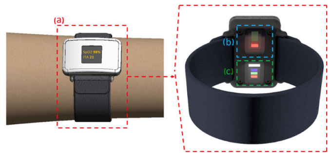
Fig. 1. Watch-type oximeter with the function of skin-color calibration.
