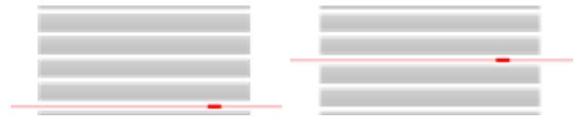
Fig. 6. Structures of carbon composite samples with FBG sensor embedded close to the surface of the laminate (left) and along its neutral axis (right).
