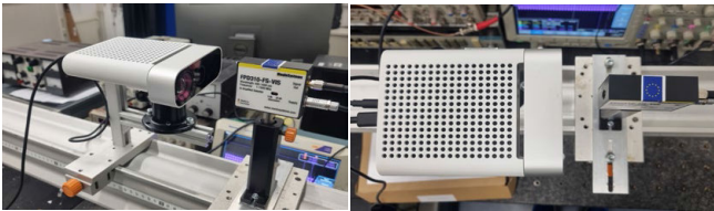
Fig. 6. Experimental setup for the assessment of the illumination system using a fast photodetector aligned with the camera.
