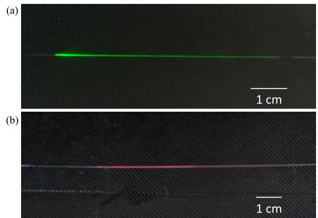
Fig. 5. Photograph of the D-fiber excited with laser lights in (a) green region, i.e., at a wavelength of 532 nm, and (b) red region, i.e., at a wavelength of 650 nm.
