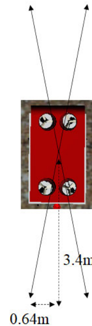
Fig. 15. Detection point by direct measurement is shown in this figure (top view of the AUV).
