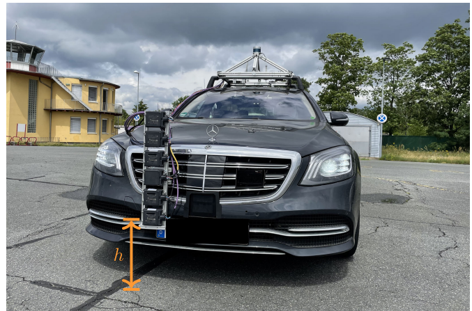
Fig. 2. Mounted sensor rack with six radar sensors at the front of the Ego vehicle. The rack has a lateral offset of 265 mm to the center. In addition to the radars and GNSS, it is also carrying lidar sensors. They are not considered in this work but the lidar data is also available within the published dataset.
