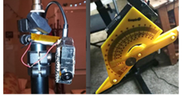
Fig. 6. Left: test bench with the AIM attached to the tripod. Right: protractor used to measure the pitch angle of the sensor system.
