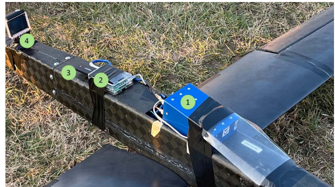
Fig. 8. Detailed view of the instrumentation placed on top of Anubi during the flight tests, performed at the Tetti Neirotti runway (Turin). (1) SmartScan interrogator. (2) Raspberry Pi 1 . (3) Internet Key. (4) Action cam. The latter was used to obtain graphic documentation of the flights.
