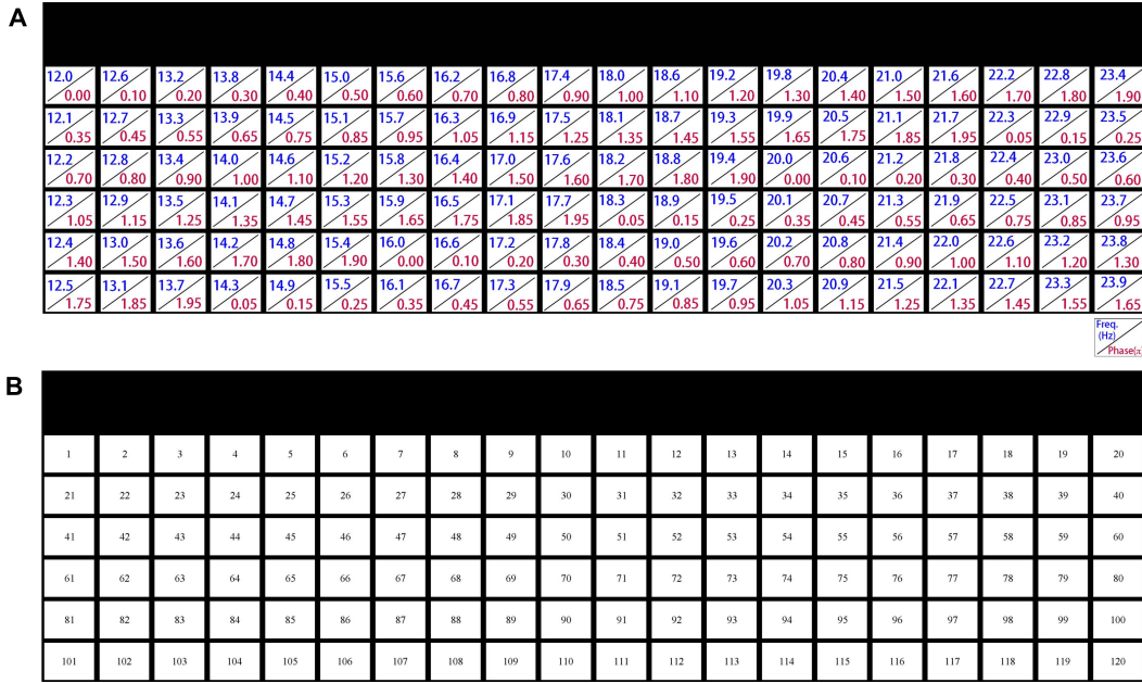
Fig. 2. Virtual keyboard for the 120-target SSVEP-BCI speller. (A) Frequency (blue) and initial phase (red) encoded by spectrally-dense joint frequency-phase modulation (sJFPM) for each stimulus. (B) User interface of the speller comprising 120 stimuli, aligned in a 6 \times 20 matrix.
