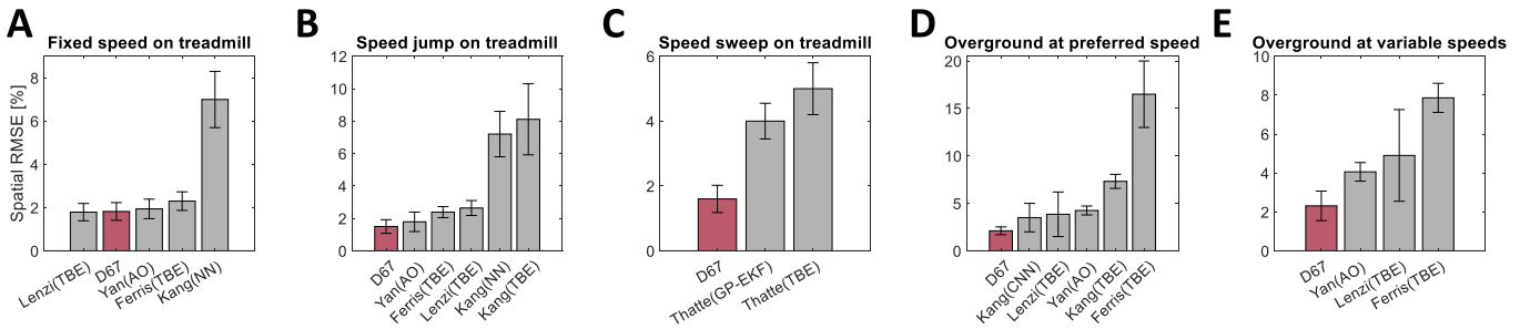
Fig. 12. Comparison of D67 gait phase estimator performance with approaches reported in the literature for (A) fixed speed, (B) speed jumps, and (C) speed sweep in treadmill walking as well as overground walking at (D) preferred speed and (E) variable speeds.
