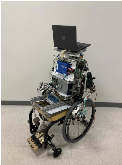
Fig. 1. The wheelchair-propelling robot used to control maneuvers in this study.
