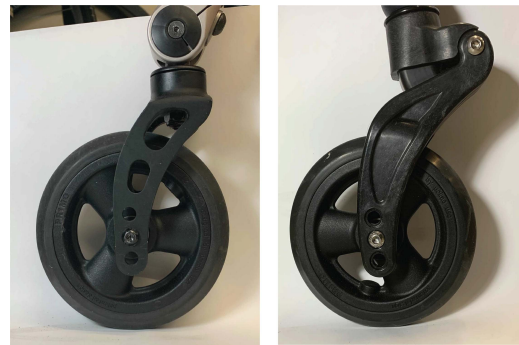
Fig. 3. (Left) Default rigid aluminum and (right) Frog Legs suspension caster forks.
