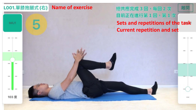
Fig. 11. Exercise window. Information includes the angles measured by the IMUs, the hold time, the remaining sets, and the number of repetitions. A video demonstration is also provided to ensure that the patient performs the exercise correctly.
