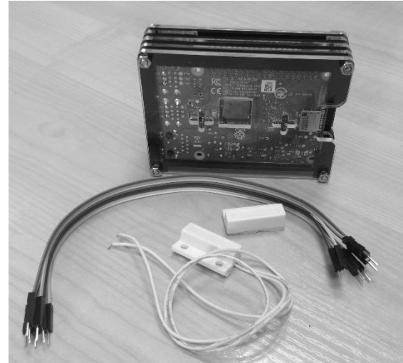
Fig. 2. Components used in the experiment: a Raspberry Pi, door sensors and cables.
