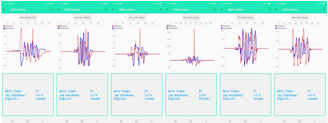
Fig. 8. The EOG signal and edge inference results for the same trial and same word, but different subjects. There is a very high inter-subject variability, indicating the biological and behavioral differences among subjects. The decoding results also indicate very robust word recognition.
