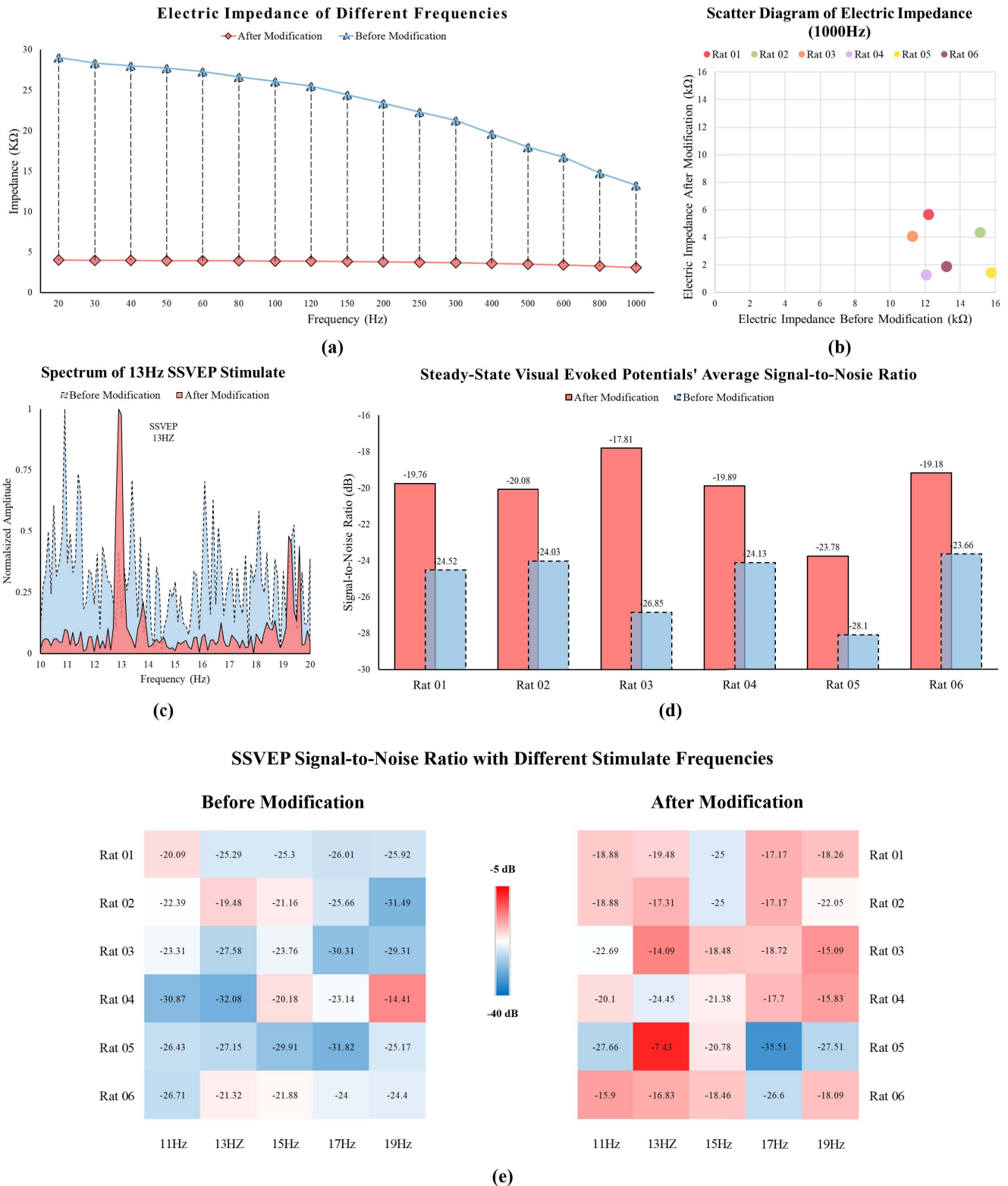
Fig. 5. (a) Shows the change of electric impedance from the ear to the modification point before and after the modification at different test frequencies, p=0.00034 . (b) shows the scatter plot of the electric impedance of each rat before and after modification when the test frequency is 1000Hz. (c) is the spectrum of EEG signal recorded by Rat 02 at the stimulation frequency of 13 Hz, and the amplitude has been normalized for facilitate comparison. (d) is the average SSVEP broadband signal-to-noise ratio of all six rats before and after modification, p=0.0008 . (e) is the heat map of SNR results for each rat at each stimulate frequency.
