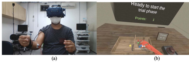
Fig. 5. (a) Volunteer using immersive VR platform using HTC VIVE Pro with EMG signal processing controller and tactile feedback. (b) the training protocol with serious games tasks and virtual prosthesis controlled by the user.
