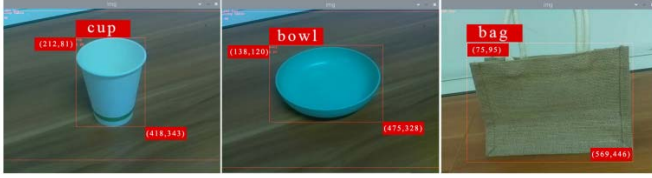
Fig. 4. Visual information from the camera and the recognition results of object category and coordinate.
