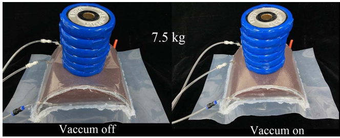
Fig. 4. When the vacuum is off, the LJS shell has low bending stiffness. When the vacuum is on, the structure has high bending stiffness. Calibrated dumbbells (1.25 kg for a single dumbbell) are used to test the load capacity of the LJS shell.
