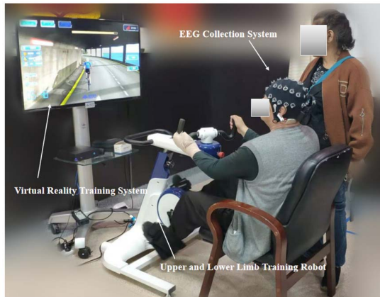
Fig. 2. The structure of the rehabilitation training system.
