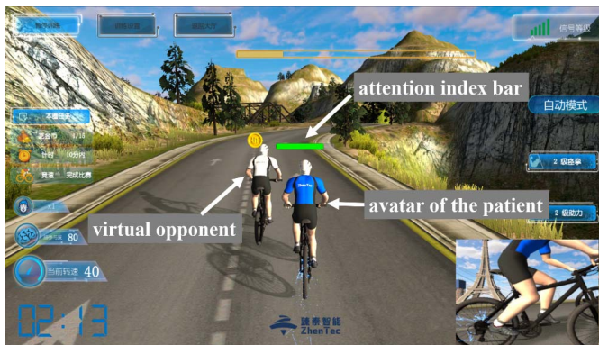
Fig. 3. Interactive screen of BCI-controlled pedaling training system during training.
