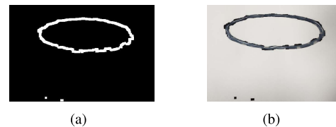
Fig. 6. Follow-up processing of Fig. 4(b). (a) Thickened contour after dilation operation. (b) A raised line map made by hand with thermoplastic material.
