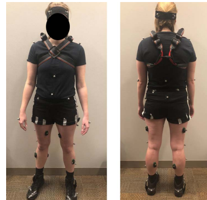
Fig. 2. Example sensor and marker setups for one subject with wireless accelerometer/sEMG sensors and motion capture markers. Subjects wore a chest harness as part of a safety system for the treadmill.
