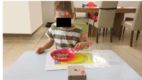
Fig. 1. Experimental setup showing the table with the plate and spoon. The sensors were placed on the spoon (B), forearm (C), upper arm (D), and head (E) and located near the transmitter (A).
