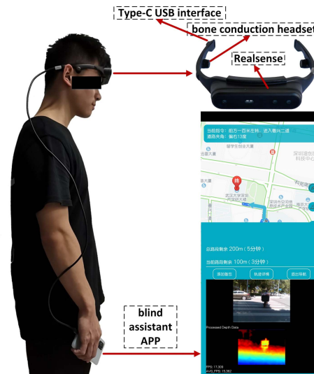
Fig. 2. The head-mounted assistive device for the blind (SensingAI G1): an RGB-D camera, a bone conduction headset, and a blind assistant app integrates the proposed system and GPS navigation.
