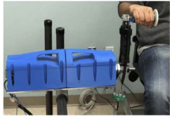
Fig. 1. The Haptic TheraDrive, a one degree-of-freedom rehabilitation robot system used in this study. Image used with permission from [38].
