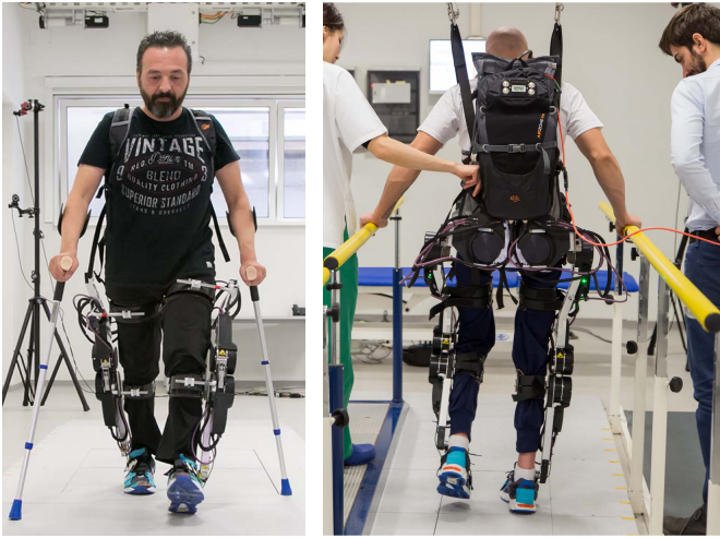
Fig. 1. SCI test pilots using the modular exoskeleton in knee-ankle configuration (KA) on the left and hip-knee-ankle configuration (HKA) on the right.
