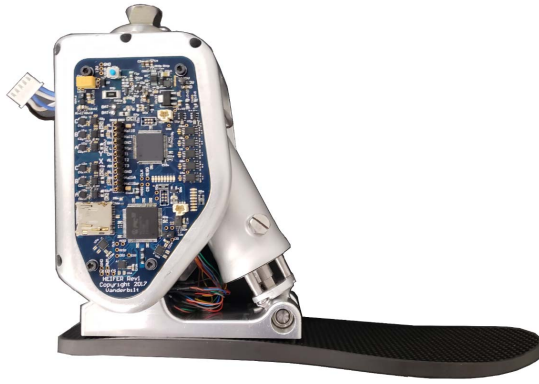
Fig. 2. Assembled semi-powered prosthetic ankle. The ankle utilizes an inverted slider crank structure and the constant volume power asymmetric actuator. The ankle joint is in series with a custom carbon fiber foot plate. The custom embedded system is visible on the side of the ankle.
