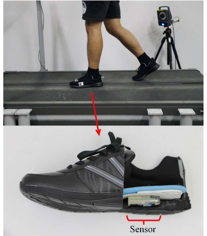
Fig. 3. Subject instrumentation layout. Reflective markers were placed on the left shoe above the calcaneus, the head of second metatarsal, and the head of fifth metatarsal. A magneto-IMU sensor was embedded in the sole of the left shoe.
