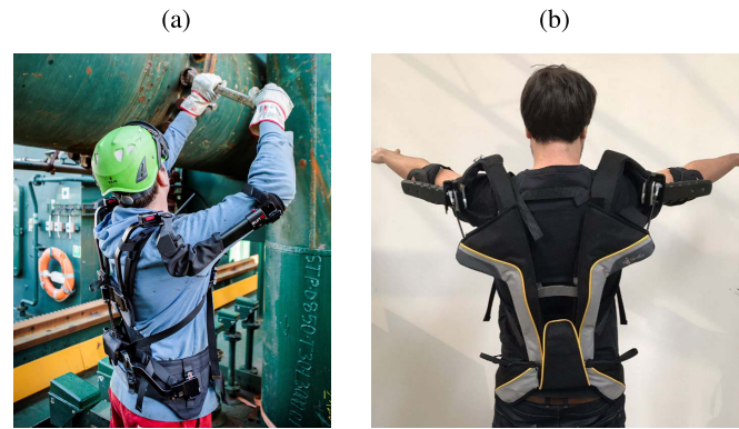
Fig. 1. The shoulder exoskeletons evaluated during this study were (a) ShoulderX V2 (SuitX, Emeryville, United States) and (b) Skelex V2 (Skelex, Rotterdam, The Netherlands). Both exoskeletons are attached to the pelvis and the upper arms. Shoulder straps ensure a stable location of the devices on the operator's body. SuitX and Skelex gave consent to illustrate both exoskeletons with pictures.
