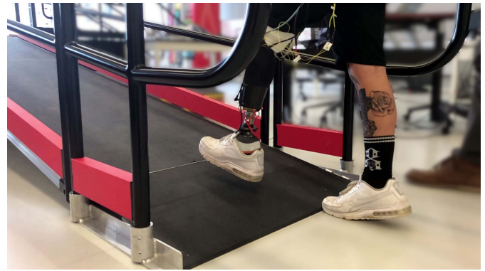
Fig. 1. Subject with TT amputation walking with the Adaptive Ankle, dorsiflexed from its neutral angle for ramp ascent. For the experiment, subjects wore their prescribed socket and customary footwear.
