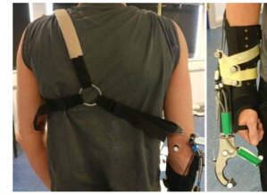
Fig. 2. TRS body-powered prosthesis simulator. Please note that these images were taken during pilot testing and as such contain additional markers not used in the final analysis.
