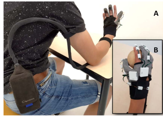
Fig. 1. Representation of instrumentation of the experiment. A) shows the entire SEM Glove™ with force sensors placed on the grey circles, B) shows the SEM Glove™ with the white inertial measurement system.
