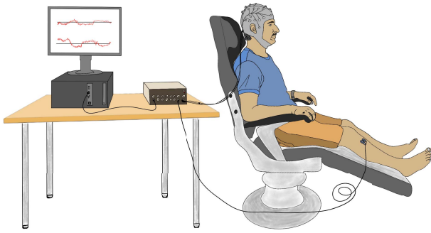
Fig. 3. An illustration of the laboratory setup for recording of EEG and sEMG data from a participant performing self-paced ballistic dorsiflexions.
