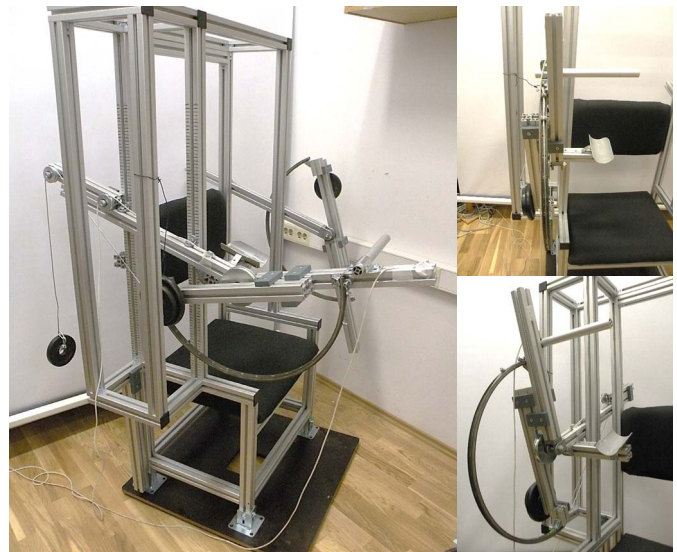
Fig. 1. Custom made brace for recording of dynamic hdEMG signals from biceps brachii muscle. The brace lever was rotatable in the sagittal plane and its torque due to the gravity was counterbalanced with counterweights. Before the measurement, additional 1 kg weight was fixed to the brace lever producing a constant torque of 3 Nm to the subject's dominant hand.
