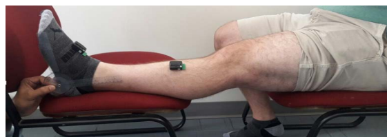
Fig. 2. Initial ankle position for measuring ankle ROM.
