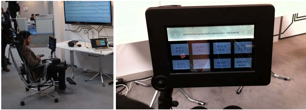
Fig. 1. BCI Appliance presented at CeBIT 2012. Left picture: battery-powered Appliance and EEG amplifier mounted on a chair, with signal displayed on the big screen for demonstration via wireless connection. Right: display of the Appliance during a spelling task. Symbols are rendered dynamically on the LCD screen, while the flickering of each field is controlled separately by underlaid LEDs.
