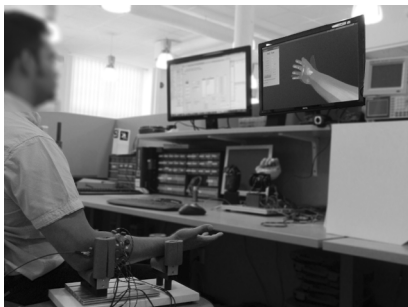
Fig. 1. Illustration of a subject performing the TAC test. Target posture shown by the shadow hand was supination, while the solid hand is controlled by the subject. Location of eight bipolar surface electrodes around the most proximal third of the forearm can be observed. Videos comparing individual and simultaneous control are available at the BioPatRec project online site [23].
