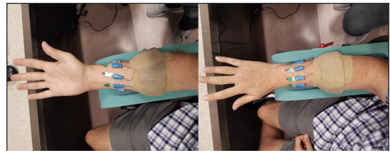
Fig. 1. Electrode Placement. sEMG data is collected using 8 Delsys Trigno sEMG sensors uniformly spaced around the right forearm.
