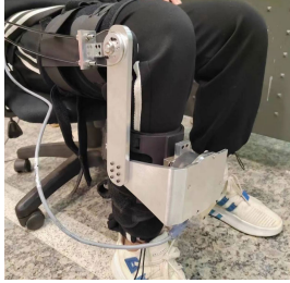
Fig. 10. Traditional unicentric knee exoskeleton.
