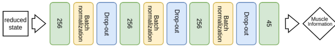
Fig. 3. Muscle prediction network. The green blocks are the fully-connected layers (indicating the number of units); the yellow blocks are the batch normalization; the blue blocks are the drop-out regularization.
