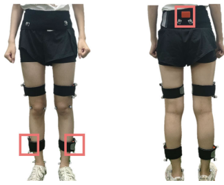
Fig. 2. Subject instrumentation layout with each orange box representing one IMU. Three IMUs were attached to each subject on the pelvis and shanks, with one IMU per segment. Four 3-marker clusters were used for motion tracking to calculate the ground truth for joint angles placed on each thigh and shank, respectively. Each shank IMU was fixed together with a 3-marker cluster.
