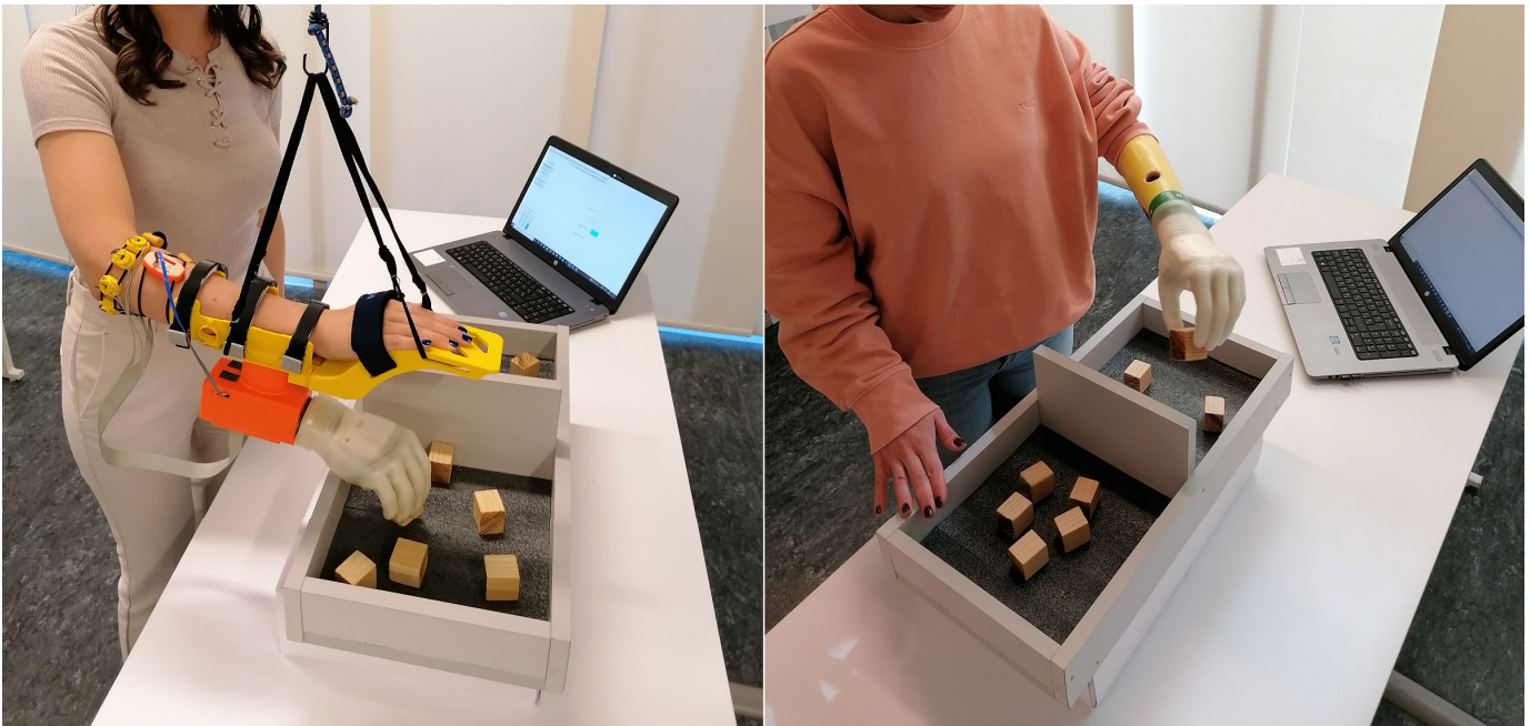
Fig. 1. The experimental setup used in non-disabled subjects (left) and in amputee subjects (right). (Left) The subject placed his/her forearm in a 3D-printed splint, with a Michelangelo prosthesis attached below. Two EMG electrodes and four vibration motors were strapped around the forearm using elastic braces. (Right) A custom designed socket, with the Michelangelo prosthesis, mounted on the subject's residual limb. Two EMG electrodes and four vibration motors, positioned equidistantly around the residual limb, were integrated into the socket. A simple graphical user interface was displayed on a laptop computer during the familiarization phase, but the screen was removed from the subjects' view when performing the main task (see text).
