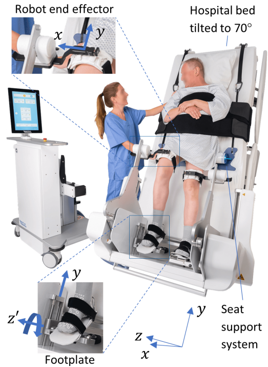
Fig. 2. VEMOTION system and setup (Reactive Robotics GmbH).
