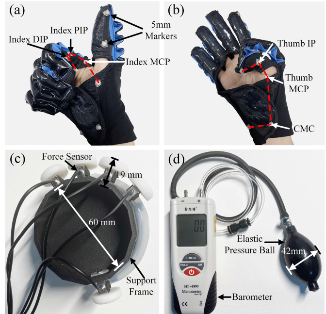
Fig. 7. Measurement diagrams and devices for finger movements and grip forces. (a) Index finger bending angle measurement diagram. (b) Thumb bending angle measurement diagram. (c) Fingertip force measurement device. (d) Finger grip force measurement device.
