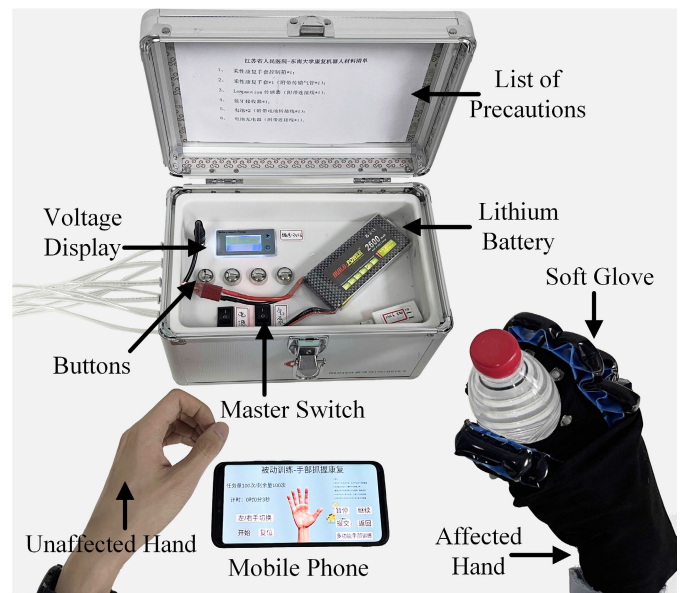
Fig. 1. Soft pneumatic glove rehabilitation system with HPAs for assisting activities of daily living.
