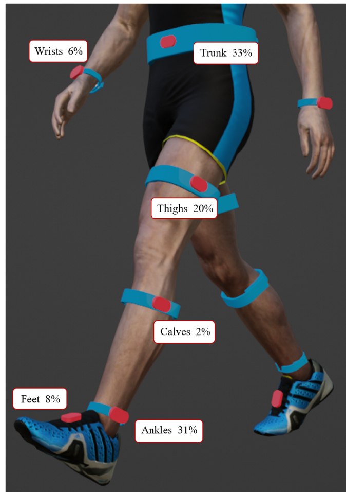
Fig. 4. The location of sensors for the assessment of PD severity and tremor based on gait.
