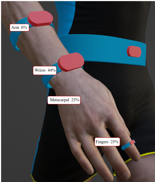
Fig. 5. The location of sensors for the assessment of PD severity and tremor based on the movement of the upper limbs.
